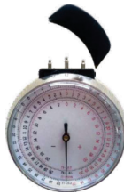
Analog Base Curve Gauge D - A12X Spec: N1.53 / 1.599 / 1.61 / 1.67
